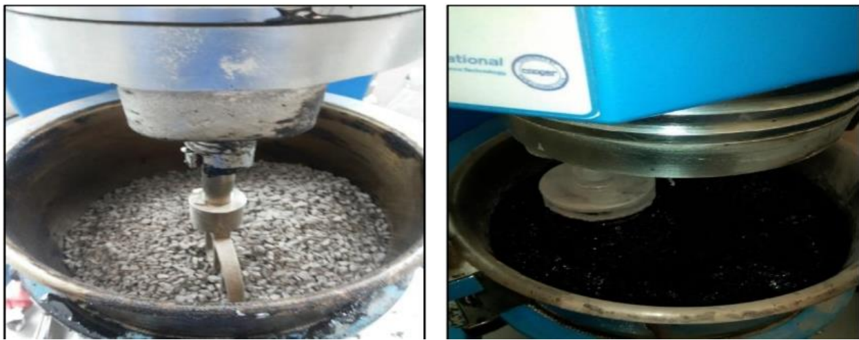
Figure 9. Mixing of asphalt materials (Lu et al., 2023)
