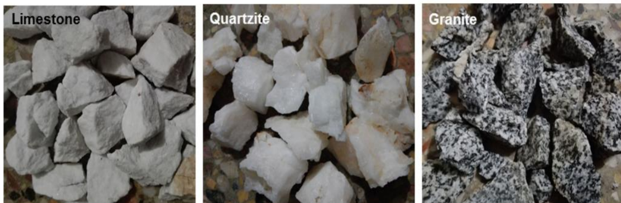
Figure (3): Coarse aggregates of Limestone, Quartzite and Granite (Tufail et al, 2016).
